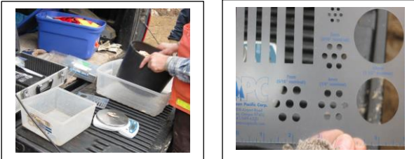
↑ On Site Chip Grading Station
